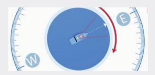
Dual antenna GNSS provides accurate heading with fast initialization time, even if the vessel is mooring.
