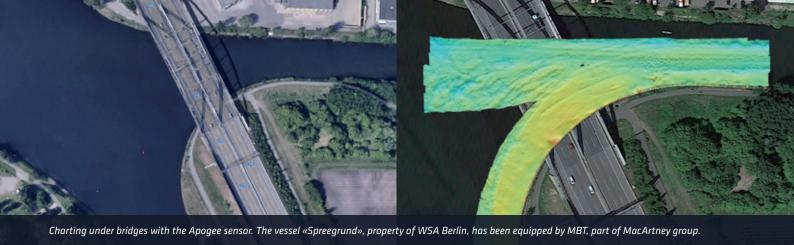
MRU or INS? Inertial Navigation Systems greatly improves navigation data in all conditions. Position information are fused in real-time with inertial data to provide a robust trajectory when GNSS outages occur (crossing a bridge, surveying a river near several mountains, etc.). In this example, the Apogee sensor is connected to an external GNSS receiver and a DVL for even better performance.
