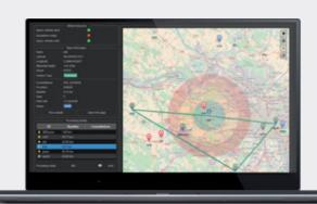
Why Post-processing? By processing all your INS and GNSS raw data forward and backward, Qinertia PPK software greatly increases accuracy, solves GNSS outages, installation errors, etc. Qinertia can save your survey, or allow you to survey in very complicated areas.
